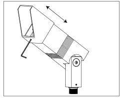
1.Use the 5/64" hex key to loosen the screw(8-32UNC set screw) on the bottom of the glare shield. Move the glare shield to the desired position, and tighten the screw ( ♠ do not overtighten).
